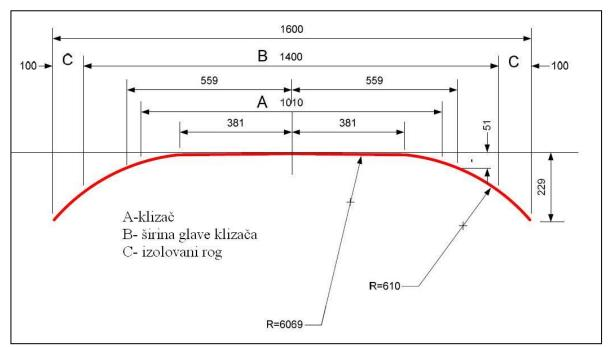
Figure No 1. – Dimensions of pantograph
